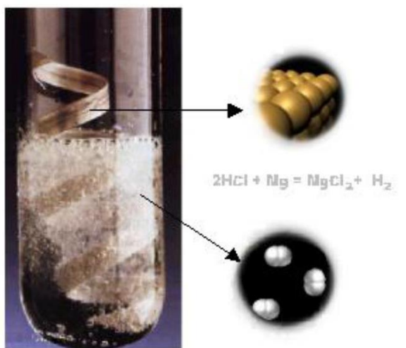
Figura 6-1 2\text{HCl}(\text{ac}) + \text{Mg}(\text{s}) \rightarrow \text{MgCl}_2(\text{ac}) + \text{H}_2(\text{g})
